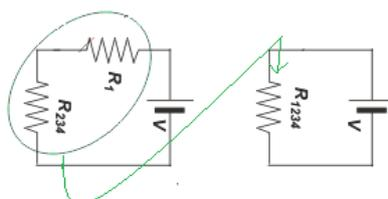
$$R_{1234} = R_1 + R_{234}$$
